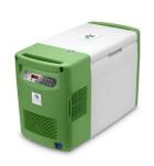
**Stirling Portable Freezers:** Stirling's ULT25NEU portable, ultra-low temperature freezer can be used to bring vaccines to remote sites at a temperature range of - 20°C to -86°C. It plugs into any 110-240V outlet, vehicle-based 12V DC power, or external battery and uses less than 2.8 kWh/day at -80 Celsius. The freezer is available with optional SenseAnywhere technology, which combines wireless sensors and secure cloud storage to remotely monitor and track temperatures.
